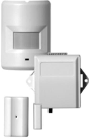
The WSK-24 Wireless Occupancy Solution automatically controls HVAC equipment by determining when a room is occupied. The WSK-24 uses the combination of an occupancy sensor and a door switch to provide optimal control. The WSK-24 is packaged in a kit that includes a 24V dry contact receiver, a wireless PIR (passive infrared receiver) occupancy sensor with mounting kit, a wireless door sensor with mounting kit, and a wiring harness.
