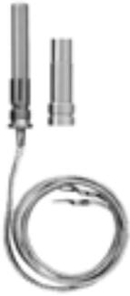
**Q313 Thermopile Generator contains multiple thermocouples connected in series to increase the millivoltage output. The power generated is sufficient to operate an automatic millivolt gas control system, independent of any outside power source.**
