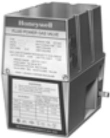
Use with V5055 or V5097 Gas Valves to control gas supply for commercial and industrial burners. Valve opens to low fire position when power is applied; valve opens all the way on demand.
