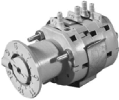
The four port, snap acting relay converts a proportional air pressure change from a controller to a positive (two-position) pressure change. It can also divert a supply line to one of two branches. Replacement device is available for Johnson, Powers, Robertshaw, Barber-Colman, and older Honeywell devices.
