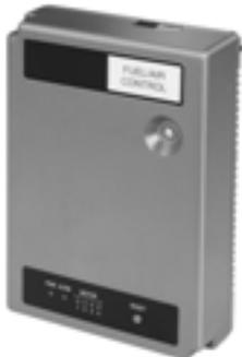
Uses microprocessor-based technology to control the ML7999 Universal Parallel Positioning Actuators. This represents a value-added replacement of mechanical cam and linkage assembly controlling the relationship between fuel, airflow and flue gas recirculation (if used) on a power burner. The ControlLinks Fuel Air Control System consists of the R7999 Fuel Air Controller, Q7999 Wiring Subbase, ML7999 Universal Parallel Positioning Actuator and ZM7999 Configuration Software. The R7999, with one
