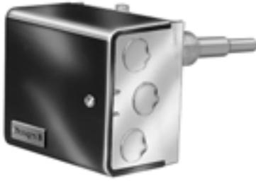
The L4103A,B is an immersion-type controller for oil-fired water heaters. The Aquastat® Controller senses water temperature and cycles the burner through the oil primary. The high-limit controller breaks the circuit to the burner on a temperature rise past the factory-set setpoint. The L4103C is an immersion-type controller for gas systems that provides water temperature regulation. The high-limit controller breaks the circuit to the burner on a temperature rise past the factory-set setpoint.
