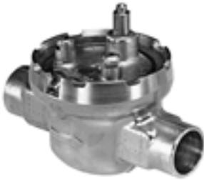
Two-way Fan Coil Valves, the VU53 high pressure zone valves are used to control the flow of hot or chilled water in commercial HVAC equipment such as fan coil units, terminal reheat coils and convectors. **IMPORTANT** These valves are not for use in systems containing dissolved oxygen.
