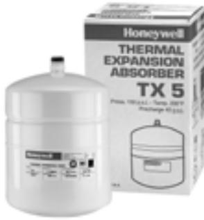
The Honeywell Thermal Expansion Absorber is a welded, pressurized expansion tank with a butyl diaphragm to control excess pressure in potable hot water systems. The Thermal Expansion Tank controls pressure build-up in the system, eliminates relief valve spillage, protects fixtures and extends water heater life.
