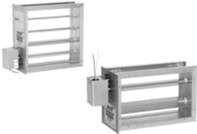
The ZD is a power close and spring open damper. It has a 24-volt motor used to control circulating air in heating, cooling and ventilating systems. It is used when a normally-open damper is required. The ZD is typically used with the TrueZONE systems and other electronic zoning systems.
