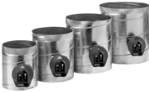
The TrueZONE® Bypass constant pressure regulating damper (CPRD) is a round static pressure relief damper. It is used in forced-air bypass applications to relieve excess static pressure when some of the zone dampers are closed.
