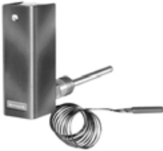
**L8100A,B, and C are immersion type controllers for regulating and limiting the tank temperature in water heaters. As the water temperature rises past the setpoint, the controller switches off the gas valve.**
