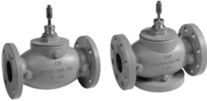
VGF Flanged Globe Valves are used for 2-position or modulating control of steam, hot water, or chilled water-glycol solutions up to 50 percent concentration in closed loop heating, ventilation and air conditioning (HVAC) systems. They can be operated by ML6984/7984, ML6420/6425, ML6421/7421 Electric Linear Actuators, MP953 Pneumatic Actuators, Modutrol™ Motors with Q5001 valve linkage, or MN/MS Series Direct Coupled Actuators with Q5020 or Q5022 valve linkages.
