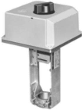
Direct Coupled Globe Valve Actuators provide floating or modulating control of chilled water, hot water, or steam, and mount directly on VGF series, V5011, and V5013 valves. These Non-Spring Return High Force Actuators will operate 1-1/2 to 6 inch valves.
