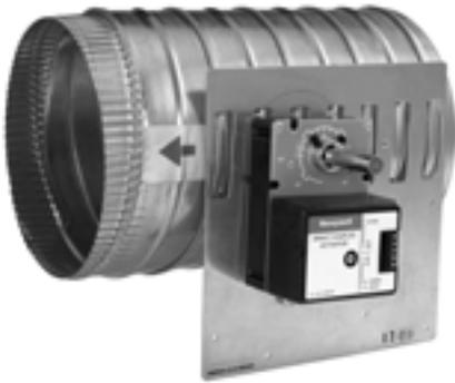
The DM7600 Commercial Zone Damper is used in zoning systems to control airflow in a round duct. A Honeywell ML6161 or ML7161 Direct Coupled Actuator is factory mounted to the damper to simplify field installation.
