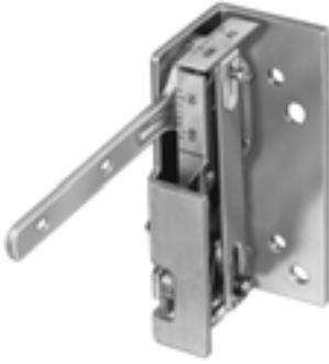
One-pipe, single temperature, low-capacity pneumatic thermostat used to provide proportional control of pneumatic valves and mixing boxes in heating and air conditioning systems. It mounts in a slot or light troffer diffuser or a return air grill.
