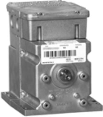
Series 62 Modutrol IV™ Motors are spring return floating control motors used with controllers that provide a switched spdt or floating output to operate dampers or valves. These motors also have an internal electrically isolated feedback potentiometer that provides indication of the motor shaft position and can be used for slaving Series 90 motors or rebalancing an external control circuit.
