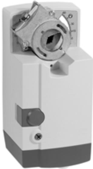
The MN7234 is a 300 lb-in (34Nm), non-spring return, direct-coupled, low voltage actuator that accepts adjustable modulating (0/2-10 Vdc) control for: air dampers, air handling units, ventilation flaps, louvers, and ball valves.
