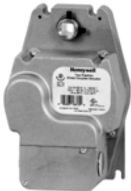
Spring return direct coupled actuators (DCA) for on/off damper control with an integral junction box. The actuator accepts an on/off signal from a single-pole, single-throw (SPST) controller. They are designed to operate reliably in smoke control systems requiring Underwriter's Laboratories Inc. UL555S ratings up to 350 F.
