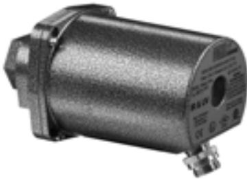
The S550B/BE is a UV/IR viewing head/flame detector. It monitors the UV and IR components and has two displays, quick disconnect plug, or pipe fitting connection, UV and IR gain settings, IR high pass filter selection, flame on/off settings and a NEMA 4X/IP67 enclosure rating.
