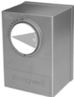
Provides 100 lb-in. torque, pulse-width-modulating (PWM) control of combustion air dampers, butterfly gas valves, oil modulation valves, and flue gas recirculation systems. The actuator includes a precision feedback potentiometer and integral power supply. The ML7999A Actuator is part of the ControLinks Fuel Air Control System, and must be used with the R7999 Fuel Air Controller.
