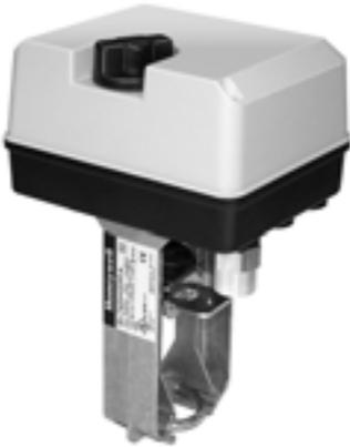
Direct Coupled Globe Valve Actuators provide floating or modulating control of chilled water, hot water, or steam, and mount directly on VGF series, V5011, and V5013 globe valves from 1/2 to 3 inches.
