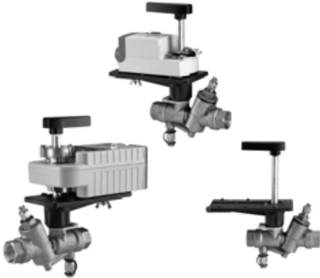
The VRN2 two-way dynamic pressure-regulating control ball valves maintain constant flow of hot or chilled water in closed loop heating, ventilating, and air conditioning (HVAC) systems regardless of head pressure fluctuations above the minimum specified pressure drop. These valve assemblies can be used with Honeywell non-spring return or spring return direct coupled actuators (DCA) with minimum torque of 35 lb-in (4 Nm) on valve sizes up to 3 inches (DN80).
