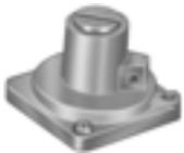
Servo gas pressure regulator for add-on or replacement use on Honeywell V400, V800, VR400, VR800 and VR8440 Combination gas controls. Utilizing the servo principle of operation, it controls burner manifold pressure by repositioning the main valve diaphragm.
