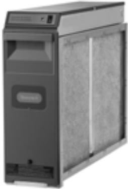
Capturing up to 98% of particles (3.0 - 10.0 micron) that pass through the filter, the F300 offers a level of filtration among the highest. It is widely compatible, operating with all gas, oil and electric forced warm air furnaces and air-conditioning systems, and is also available in four convenient sizes to fit most ducts.
