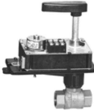
The VBN3 Three-Way Control Ball Valves control hot and chilled water with glycol solutions up to 50% in heating, ventilating, and air conditioning (HVAC) systems to provide two-position or modulating functions. These valve assemblies can be ordered with or without factory-mounted non-spring return or spring return direct-coupled actuators (DCA).
