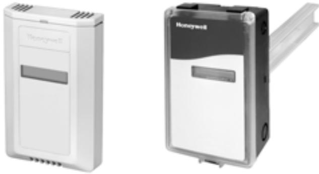
The Carbon Dioxide (CO<sub>2</sub>) Sensors and Controllers are stand-alone carbon dioxide (CO<sub>2</sub>) sensors for use in determining ventilation necessity with HVAC controllers. The sensor measures the CO<sub>2</sub> concentration in the ventilated space or duct. The sensors are used in ventilation and air conditioning systems to control the amount of fresh outdoor air supplied to maintain acceptable levels of CO<sub>2</sub> in the space.
