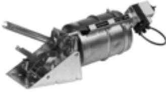
Used for proportional control of medium- to large-size dampers in HVAC systems. The MP918A,B are rolling diaphragm, piston-type actuators. The MP918A has a positive positioner. Replacement devices are available for Johnson, Powers, Robertshaw, Barber-Colman, and older Honeywell actuator models.
