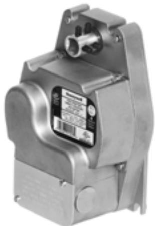
The MS8309F is a 80 lb-in (9Nm), spring return direct-coupled, 24 Vac, CCW actuator that accepts two position (SPST) control with an integral junction box. The actuator accepts an on/off signal from a single-pole, single-throw (SPST) controller. They are designed to operate reliably in smoke control systems requiring Underwriter's Laboratories Inc. UL555S ratings up to 350 F.
