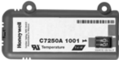
**The C7250 Mixed Air sensor is designed for use as a 20k input to a controller for mixed air temperature in rooftop packaged air conditioning equipment.**
