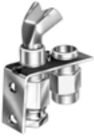
**Non primary-aerated, insert orifice type pilot burner for main burner ignition. Used with Q309, Q340, and Q390 thermocouples or Q313 thermopiles.**
