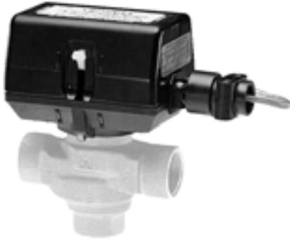
Control central heating and/or cooling systems, fan coil systems, radiators and convectors. Depending on the model selected, it can be controlled by either a low or line voltage SPST or SPDT or floating or modulating controller such as a room thermostat, Aquastat control, flow switch or a 0/2 to 10 Vdc controller.
