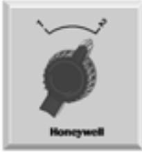
Pneumatic diverting switch used to manually divert, block, or bleed air in pneumatic air lines to revise control sequence with a change in conditions. Commonly applied on Day-Night, Summer-Winter, On-Off-Auto, or Start-Stop functions. Replacement kits are available for Johnson, Powers, Robertshaw, Barber-Colman, and older Honeywell switches.
