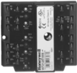
W7212, W7213, and W7214 Economizer Logic Modules are used with CO2 Demand Control Ventilation (DCV) Sensors, and solid state C7400A Enthalpy Sensors or C7660 Dry Bulb Temperature Sensors. All models proportion outdoor and return air dampers for control of free cooling in commercial HVAC equipment.
