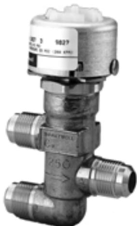
Three-way pneumatic mixing valve provides proportional control of hot and/or cold water in unit air conditioners and fan coil systems. Replacement devices are available for Johnson, Powers, Robertshaw, Barber-Colman, and older Honeywell devices.
