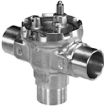
**Three-way Fan Coil Valve, the VU54 high pressure zone valves are used to control the flow of hot or chilled water in commercial HVAC equipment such as fan coil units, terminal reheat coils and convectors. IMPORTANT These valves are not for use in systems containing dissolved oxygen.**
