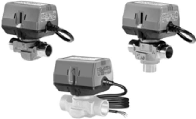
Control central heating and/or cooling systems, fan coil systems, radiators and convectors. Depending on the model selected, it can be controlled by either a low or line voltage SPST or SPDT or floating controller such as a room thermostat, Aquastat control, or flow switch.
