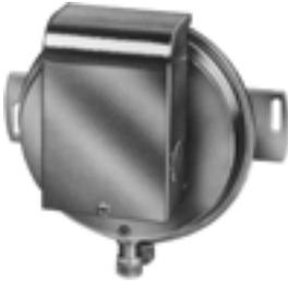
Airflow Differential Pressure Switches are used to sense positive, negative, or differential air pressure in HVAC systems. They provide high or low limit with alarm or high limit shutdown with manual reset.
