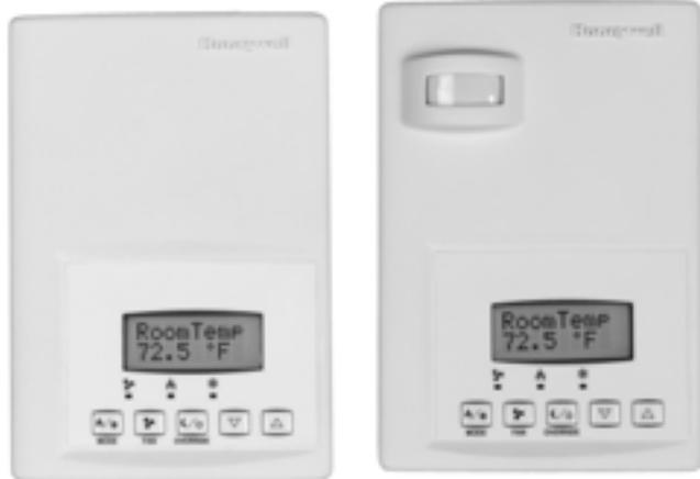
Select from a range of 24 Vac models that provide control of 2 or 4 pipe fan-coil units with on/off, floating or analog control and manual or automatic heat/cool changeover. Additionally, 3-speed fan control and auxiliary on/off heat control with relay (not included) are also supported. All models include a remote sensor input, two digital inputs, universal input, and an auxiliary output.
