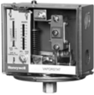
Provide operating control and automatic high limit protection for vapor heating systems with pressures up to 4 psi (8 kPa). All models have MicroSwitch snap switches to open or close a circuit on a pressure rise.
