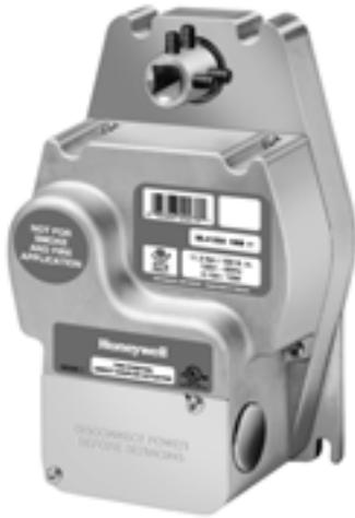
The ML8125 Fast-Acting, Two-Position Actuators are spring return direct coupled actuators (DCA) with an integral junction box for on/off damper control.
