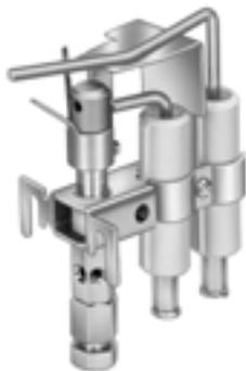
**Q179A,B Gas Pilot Burner Assemblies use the flame rectification principle to prove the flame. Q179A,B are used in conjunction with a suitable electronic flame safeguard control on industrial or commercial gas and gas pilot ignited oil burners.**
