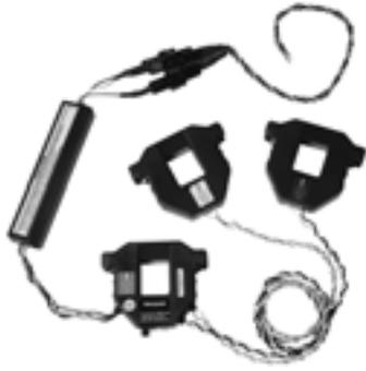
The Honeywell SXB40/SXB50 Series kW (real power)/kWh (consumption) transducers combine processing electronics and industrial grade current sensors in an easy-to install split-core package. These devices continuously measure voltage and current values for the monitored conductors and update calculations to provide highly accurate true RMS power readings. Models designed for balanced loads include one current sensor only, while models for unbalanced loads have three current sensors.
