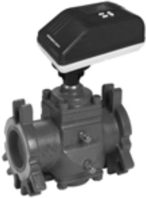
The VRW2 two-way dynamic pressure-regulating control valves maintain constant flow of hot and chilled water in closed-loop heating, ventilating, and air conditioning (HVAC) systems regardless of head pressure fluctuations above minimum specified pressure drop. These valves come complete with proportional, stay-in-place or electronic fail-safe actuators.
