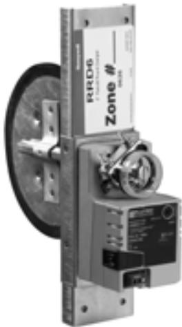
The RRD is a round damper that is easily inserted into rigid round ducts for retrofit zoning in forced air heating and cooling systems. It is available in four sizes for use in 5 in., 6 in., 7 in., and 8 in. ducts. The damper is used with Honeywell HZ221, HZ311, HZ322, HZ432 and similar zone control systems. The power open, power closed actuator draws 2 VA allowing multiple dampers per zone, but delivers high torque for reliable operation.
