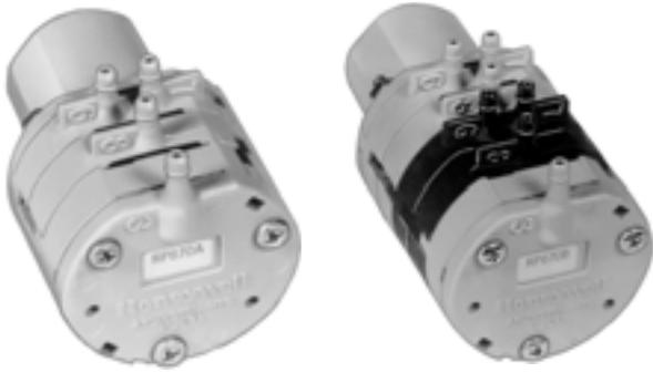
Pneumatic switching relays block, divert, or bleed pneumatic air lines when pilot pressure is changed from one specific value to another. Commonly applied in Day-Night, Summer-Winter, Start-Stop, On-Off-Auto and other multiple condition systems where control sequence is changed as conditions change. Replacement devices are available for Johnson, Powers, Robertshaw, Barber-Colman, and older Honeywell devices.
