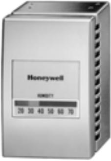
A proportioning pneumatic humidistat used on one- or two-pipe installations for controlling actuators on valves and dampers in air conditioning systems for humidification or dehumidification control.
