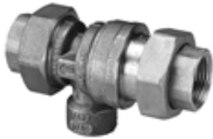
The BP900 is a double check backflow preventer with an intermediate vacuum breaker designed to prevent the backflow of contaminated water into the potable water supply. Designed for the use on small supply lines, it protects against both backflow and back siphonage for continuous pressure applications.
