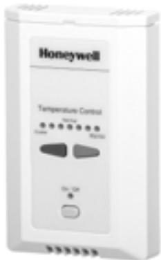
The T7771A Remote Temperature Sensors are direct wired wall modules for use with the Honeywell T7350 Commercial Programmable Thermostat. The T7771A has a space temperature sensor, LED push button setpoint adjustment, and override with LED.
