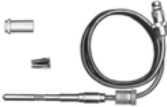
Thermocouples generate a thermoelectric current that senses a pilot flame on gas-fired heating systems. The pilot flame heats the tip of the thermocouple, producing a temperature differential between it and the base. This temperature difference generates a small amount of DC power, measured in millivolts.
