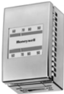
One- or two-pipe, single temperature, low capacity, pneumatic thermostat used to provide proportional control of pneumatic valves and damper actuators in heating and air conditioning systems. Replacement kits are available for Johnson, Powers, Robertshaw, Barber-Colman, and older Honeywell pneumatic thermostats.
