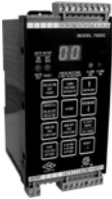
The 700 is a signal processor which amplifies and conditions the viewing head signal for use with a burner management system. It provides a 0/4-20mA output signal, two SPDT flame relay outputs and one SPDT self-check relay output.
