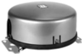
One- or two-pipe, direct- or reverse-acting, low- or high-capacity controller used with pneumatic actuators to regulate static or differential pressure in central fan installations. Replacement devices are available for Johnson, Powers, Robertshaw, Barber-Colman, and older Honeywell devices.
