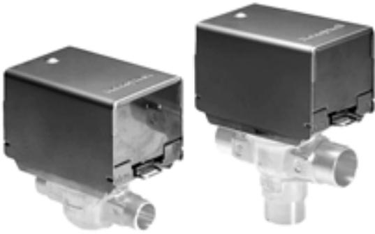
The VU844 Fan Coil Valve Actuators are used in conjunction with the VU52, VU53 and VU54 valves for controlling the flow of hot or chilled water in commercial HVAC equipment such as fan coil units, terminal reheat coils and convectors. These valves are humidity resistant and are suitable for use in condensing, non-corrosive environments.
