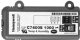
The C7400S SyLK Bus sensor is a combination temperature and humidity sensor, which is intended to be used in commercial roof top units for sensing air. The sensor is powered by and communicates on the SyLK Bus. The C7400S communicates temperature and humidity separately digitally on the SyLK Bus Communication Protocol.
