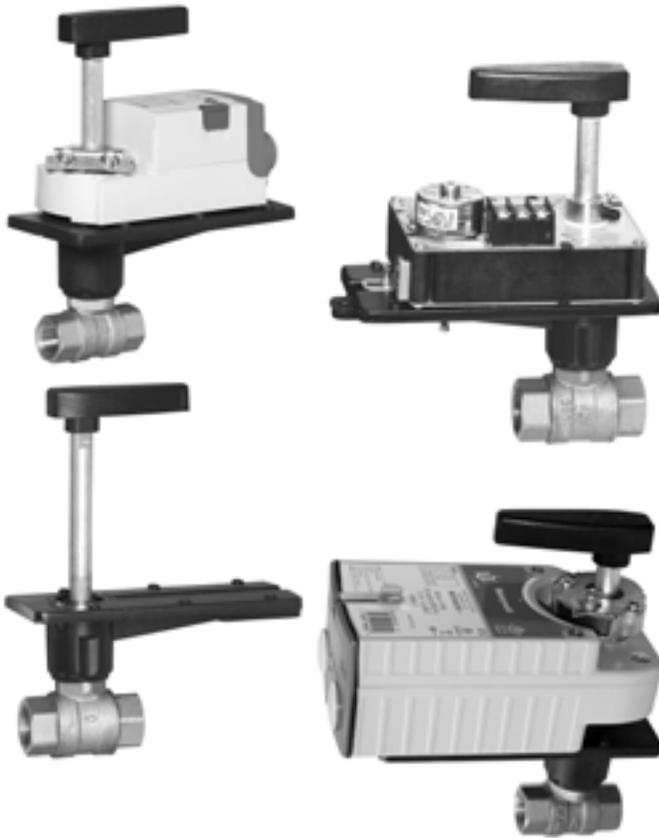
The VBN2 Two-Way Control Ball Valves control hot and chilled water with glycol solutions up to 50% in heating, ventilating, and air conditioning (HVAC) systems to provide two-position or modulating functions. These valve assemblies can be ordered with or without factory-mounted non-spring return or spring return direct-coupled actuators (DCA).
