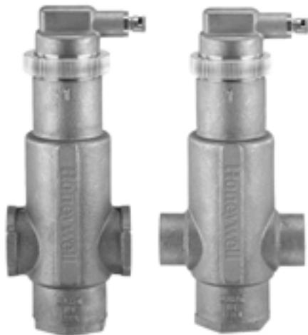
Conventional automatic air vents installed in Hydronic heating systems can leak and cause inefficient system operation. To effectively eliminate air from the system without bleeding, air bubbles need to be vented. The NEW Honeywell SuperVent purges air through a no clog vent assembly that controls dirt and debris to minimize air vent fouling.
