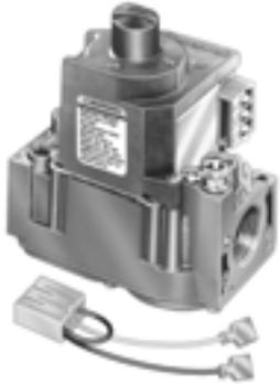
Universal electronic ignition combination gas control for use with direct spark ignition, hot surface ignition or intermittent pilot ignition in 24 Vac, gas-fired appliances, with capacities from 20 to 200 cfh (VR8245M) or 30 to 415 cfh (VR8345M).
