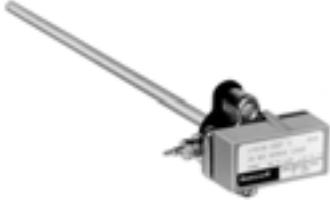
One-pipe, direct-acting temperature sensor used with RP908/ RP920 Controllers to provide proportional control of pneumatic valve or damper actuators. Rod and tube insertion element for duct, well, or through-the-wall mounting.
