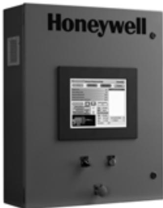
Delphi Combustion Efficiency Panel is a packaged, pre-wired panel with integrated color touchscreen display, flame safeguard control, linkageless fuel/air ratio control, oxygen trim and VFD capability. Includes Hall-effect sensor which monitors VFD-driven blower and provides feedback to the control, certain models include the MF020-1-LC3 Oxygen sensor with mounting fitting and electrical connector. System is set-up entirely via the touchscreen interface.
