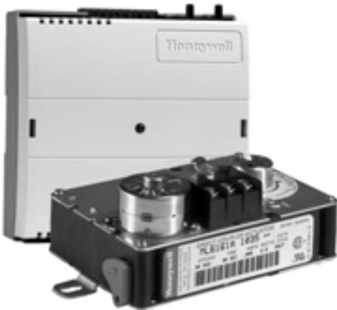
The W7751F2003 VAV II Controller is from the Excel 10 family product line. VAV controllers provide pressure independent or pressure dependent air flow control and series and parallel (induction) fan control using single and dual applications. The W7751F controllers provide additional outputs that control VAV box reheat coils. The ML6161B2024 is used to control dampers in VAV terminal units and for mounting on ball valves.
