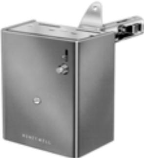
One-piece, stack-mounted oil burner primary controls that cycle the burner on and shut down the burner on flame loss or system malfunction.
