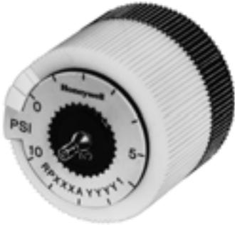
A four port non-bleed pneumatic relay which produces a modulating pressure output, proportional in a fixed ratio to pilot input changes. It is used to control pneumatic valve or damper actuators in sequence from a single thermostat. Replacement actuators are available for Johnson, Powers, Robertshaw, Barber-Colman, and older Honeywell devices.
