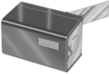
The S637 Sail Switches respond to the air velocity in heating or warm air ducts, such as used in farm crop dryers. The switch completes a 24V or line voltage burner control circuit only when the blower or fan has produced a predetermined air velocity.
