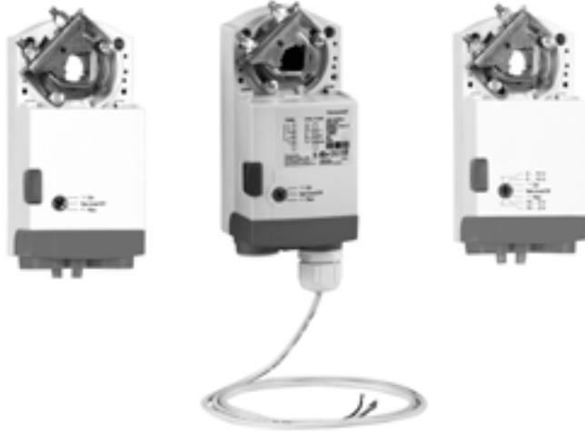
The MN7505W is a 44 lb-in (5Nm), non-spring return, direct-coupled, low voltage actuator that accepts adjustable modulating (0/2-10 Vdc) or on/off (SPDT) control for: air dampers, air handling units, ventilation flaps, louvers, and ball valves. This model includes a 3 foot whip.
