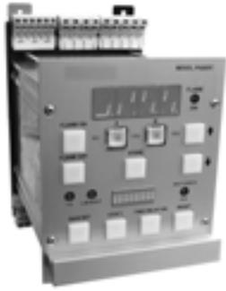
**P522 signal processors amplify and condition the viewing head signal for a burner management system. Provides 0/4-20mA output signal, 2 SPDT flame relay outputs and 1 SPDT self-check relay output. Connect 2 S55xB/BE viewing heads and channel toggle.**
