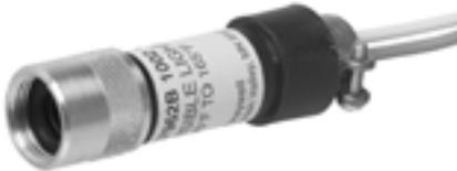
The C7962B Visible Light Flame Detector detects the visible light emitted by fuel oil combustion flames. The C7962B Detector is used with Honeywell Flame Safeguard controls to provide fuel oil flame supervision in commercial and industrial burners.
