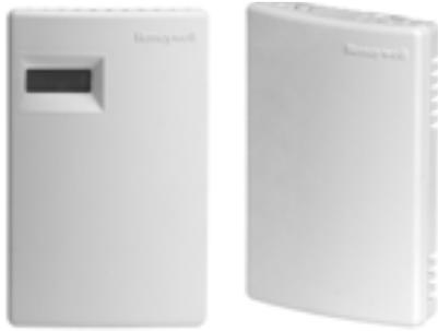
The C7262 Sensor is a stand-alone carbon dioxide (CO<sub>2</sub>) and temperature sensor for use in determining ventilation necessity with HVAC controllers. The C7262 measures the CO<sub>2</sub> concentration and temperature to control the amount of fresh outdoor air supplied to maintain acceptable levels of CO<sub>2</sub> in the space.
