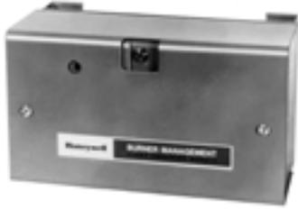
The FSP5075A Flame Amplifier Module is designed to accept a variety of Honeywell plug-in flame signal amplifiers. Depending on the plug-in amplifier model installed, the flame amplifier module can be used with ultraviolet flame detectors, infrared flame detectors, rectifying flame rods or rectifying photocells to provide
