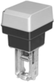
Direct Coupled Globe Valve Actuators provide floating and modulating control of chilled water, hot water, and steam, and mount directly on VGF series, V5011, and V5013 globe valves. These Spring Return Actuators will operate 1/2 to 3 inch valves.
