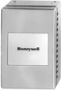
One- or two-pipe, direct-acting humidity sensor used with RP908/ RP920 Controllers to provide proportional control of pneumatic valve or damper actuators in systems requiring humidification or dehumidification control.
