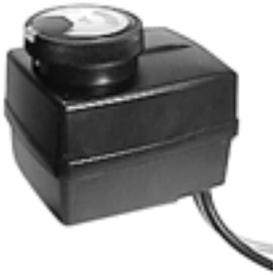
The Corona series of M6063 Actuator and V5442 Compact Rotary Valves provide integrated mixing of boiler supply, boiler return, loop supply, and loop return water in hydronic heating systems. The M6063 actuator enables automatic mixing operation when used with an AQ675A Aquatrol Outdoor Temperature Compensator, or T6984 proportional room thermostat.
