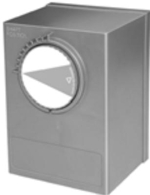
ML7999B Universal Direct Coupled Actuator provides 100 lb-in. torque, 4 to 20 mA control input to control combustion air dampers and modulation valves. The actuator includes precision drive shaft control and integral power supply capable of direct line voltage connection.
