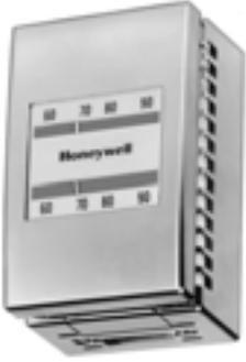
Pneumatic thermostat with night setback used to provide proportional control of pneumatic valves and damper actuators in heating and air conditioning systems. Replacement kits are available for Johnson, Powers, Robertshaw, Barber-Colman, and older Honeywell two-pipe pneumatic thermostats.
