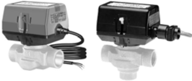
Control central heating and/or cooling systems, fan coil systems, radiators and convectors. Depending on the model selected, it can be controlled by a low voltage SPST or SPDT switch, pulse-width modulated 24 Vac signal, or floating input, modulating controller such as a room thermostat, Aquastat control, flow switch or a 0/2 to 10 Vdc controller.
