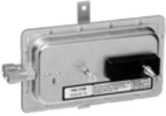
Senses differential air pressure in HVAC systems and provides an on/off output. A typical application is sensing fan shutdown in a unit ventilator to close the outdoor air damper.
