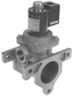
V4297S are normally open (vent) solenoid gas valves. Suitable for use on furnaces, ovens, atmospheric burners, commercial water heaters, roof-top make-up air units, power burners, and commercial/industrial boilers.
