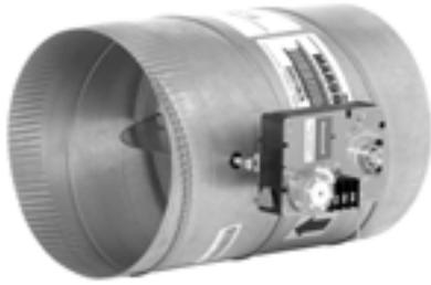
The Modulating Automatic Round Damper is a round damper with a 24-Vac, floating-control type modulating motor for bypass and zone damper control.
