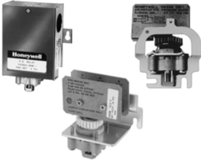
Pneumatic-electric switches (P658A,B,E and F) used to convert a pneumatic signal from a controller to an electrical switching action (SPDT) to provide start and stop control of equipment such as fans and pumps. Replacement devices available for Johnson, Powers, Robertshaw, Barber-Colman, and older Honeywell pneumatic/electric switches.
