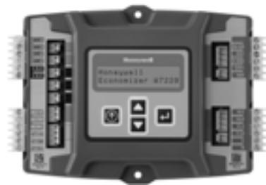
The JADE™ Economizer System is an expandable economizer control system, which includes a W7220 Economizer Module (controller) with an LCD and keypad. The W7220 can be configured for 4 different economizer strategies: referential or differential dry bulb, referential or differential enthalpy.
