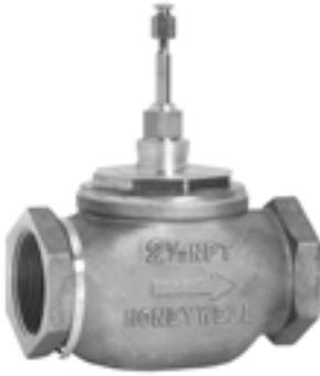
Used for two-position or modulating control of steam and water and glycol solutions (to 50 percent concentration) in heating or cooling systems.
