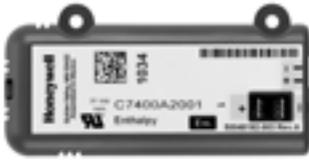
The C7400A Enthalpy Sensor is used with the economizer logic modules with the A,B,C, and D performance curves; the C7400C sensor is used with the logic modules with the A,B,C,D, and E performance curves. The sensors combined with the economizer logic modules permit the use of outdoor air as the first stage of cooling in heating, ventilating and air conditioning (HVAC) systems.
